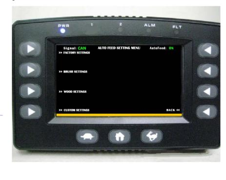
Press the soft key to the left of the >> CUSTOM SETTINGS key for the user to customize an Auto Feed setting.
