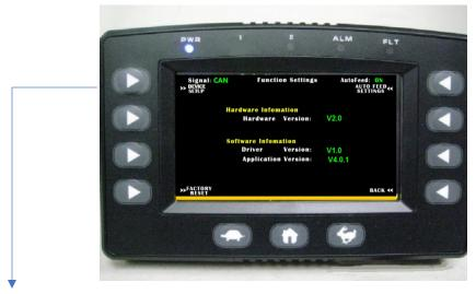
Press the soft key to the left of >>DEVICE SETUP to configure the iQView
