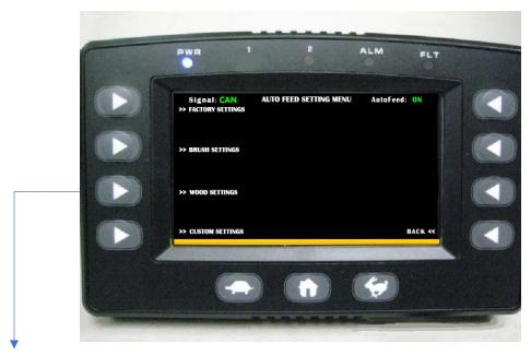
Press the soft key to the left of >> WOOD SETTINGS to customize wood chipping.
