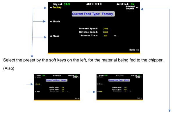
To switch the Auto Feed function ON or OFF, press the Soft Key to the right of the Auto Feed ON/OFF << prompt, which is available on all three of the current feed pages.
