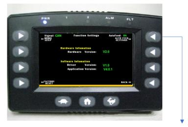
Press the soft key to the right of AUTO FEED SETTINGS to configure the Auto Feed
