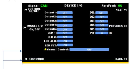
This menu is protected by a password and will lead to the password page for user input. Specific lines needing a password are found with an asterisk.
