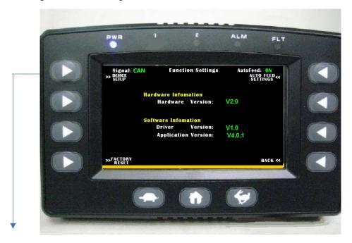
Press the soft key to the left of >>DEVICE SETUP to configure the iQView
