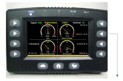
Pressing the soft key to the right of the DEVICE I/O << prompt will display the DEVICE I/O menu.
