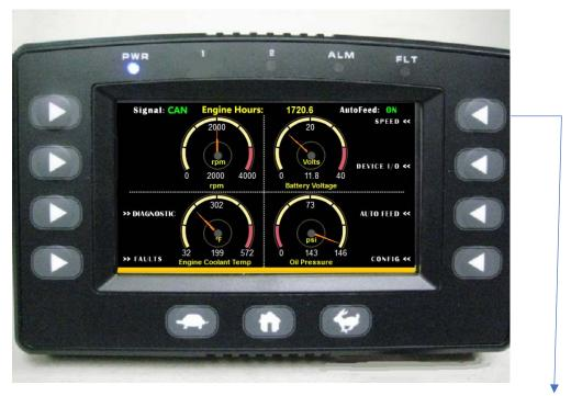
Pressing the Soft Key to the right of SPEED<< prompt will display the TARGET SPEED menu.
