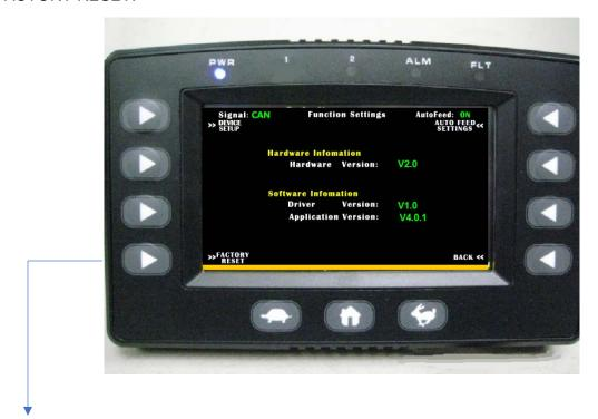
If desired or required, a full factory reset is avialible here at this soft key!
