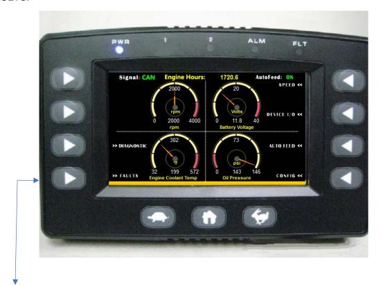
Pressing the soft key to the left of >>FAULTS will displays Faults detected on the CAN:
